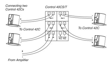
Use only two or four satellite loudspeakers as described in the recommended configurations. Failure to do so may result in uneven sound levels and / or damage to your sound system.
